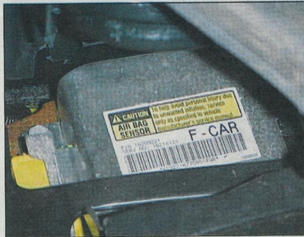
A car's "black box" can provide vital information in determining the cause of an accident.
